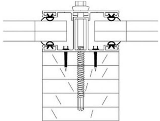
**5. OBERPROFILE MONTIEREN**
